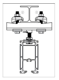
Move the screws of the clamping jaws  $\ @$  as close as possible to the overhead structure.
