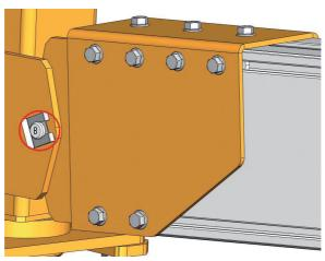
**Step 2:** Mount the anchoring to the swivel joint using the bolt.
